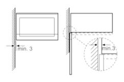
Measurements in mm
