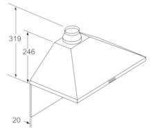
If a back panel is used, the design of the appliance must be considered.
