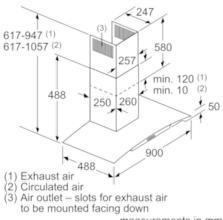
min. 550/650 electric/gas\* measurements in mm measurements in mm
