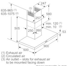
measurements in mm
