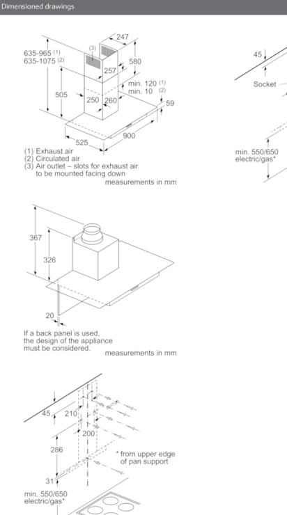
measurements in mm
