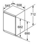
measurements in mm
