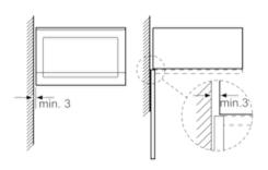
Measurements in mm
