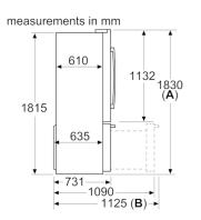
A: Front is adjustable from 1830 to 1847, with front levelling feet fully extended B: With handle
