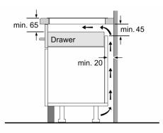
Measurements in mm
