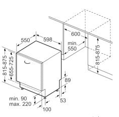
measurements in mm
