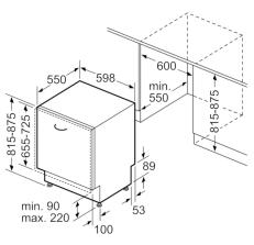
measurements in mm
