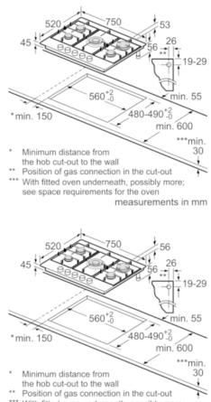
\*\* Position of gas connection in the cut-out \*\*\* With fitted oven underneath, possibly more; see space requirements for the oven measurements in mm
